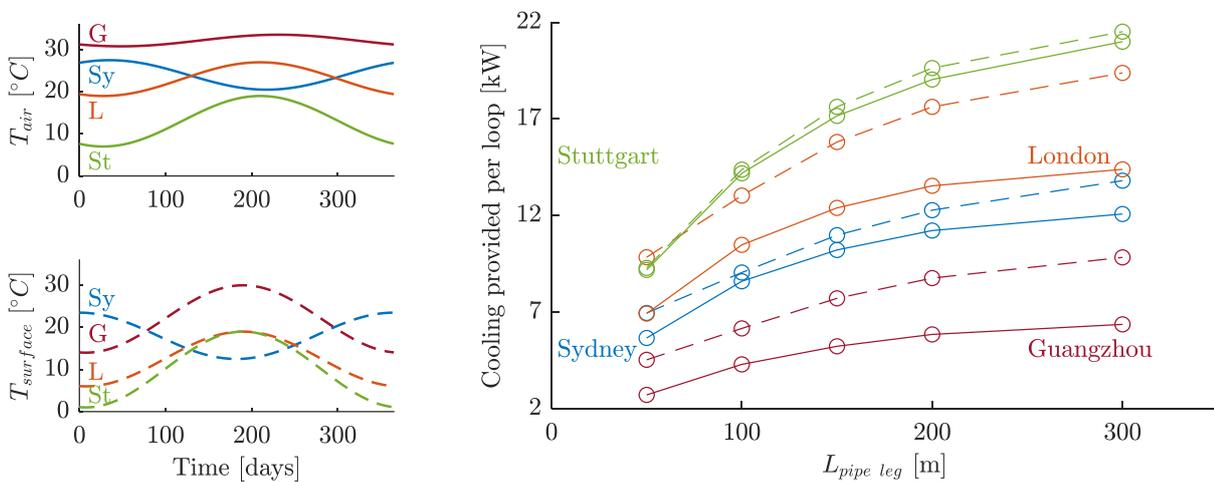
**Figure 1:** The left panel shows the air temperature distributions for the tunnel air ( $T_{air}$ ) and the surface temperature ( $T_{surface}$ ), for the four investigated locations, Sydney (Sy), Guangzhou (G), London (L), and Stuttgart (St, colour-coordinated). The resulting cooling thermal power per pipe loop that can be provided is shown (right panel) for the two entering air temperature distributions (solid:  $T_{air}$ , dashed:  $T_{surface}$ ), varying with length of activated tunnel.
