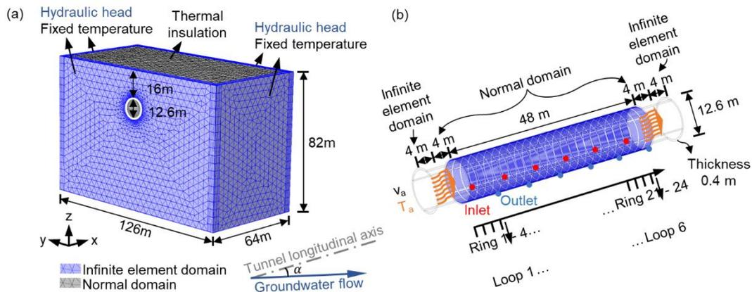
**Figure 1: Numerical model: (a) geometry, mesh, and key boundary conditions, and (b) tunnel details and heat absorber pipes.**
