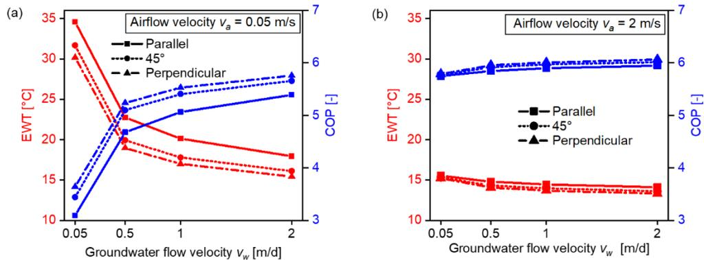
**Figure 2: Results: average entering water temperature and the COP of the GSHP for (a)  $v_a = 0.05$  m/s, and (b)  $v_a = 2$  m/s.**
