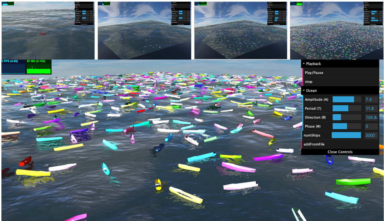
Figure 8: Simulating the seakeeping behavior of 1, 100, 1000 and 3 000 hulls using closed-form functions, in a virtual 4km x 4km ocean with virtual waves.
