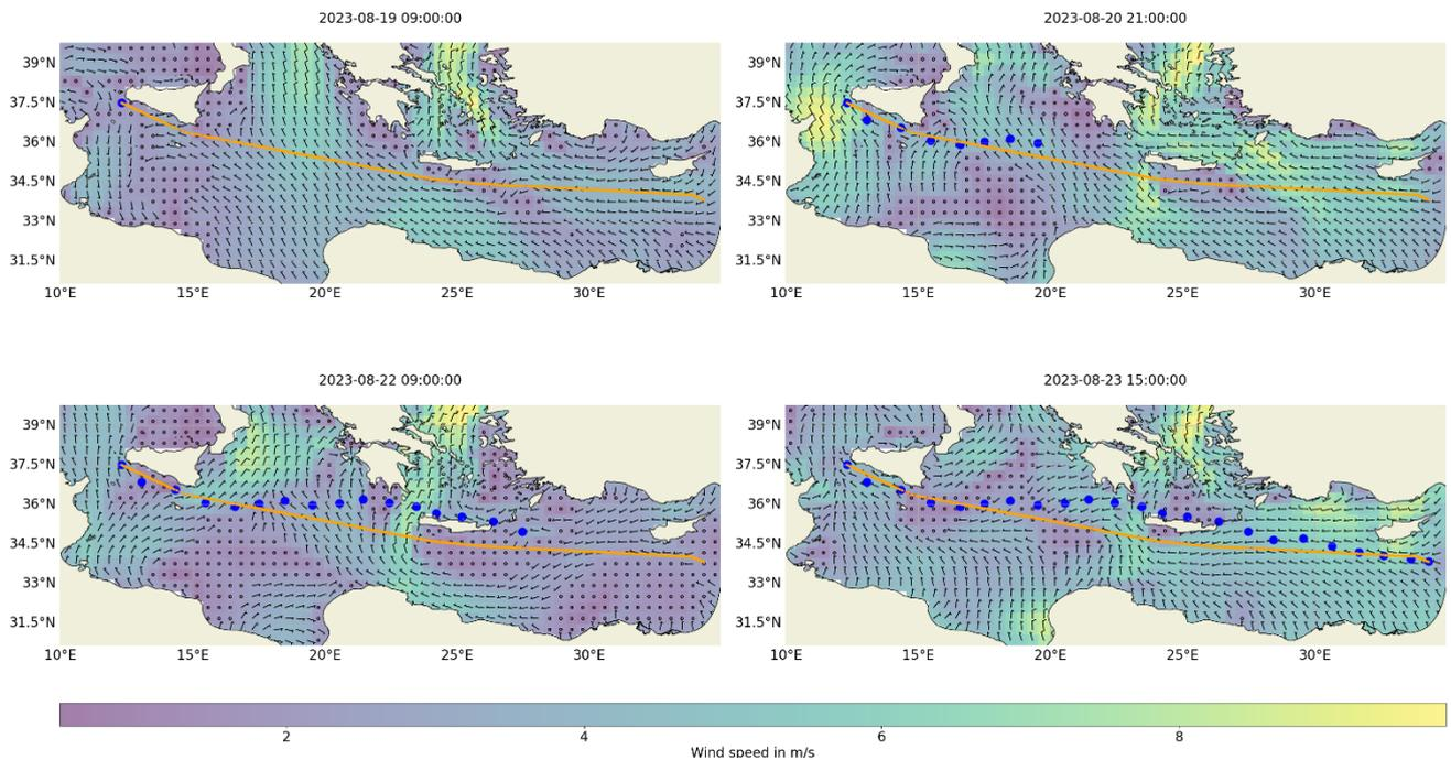
**Figure 24: Trajectories of reference (orange) and optimized (blue) routes in the Crete scenario for four snapshots. The background map shows wind speed and wind direction as heat map and wind barbs.**
