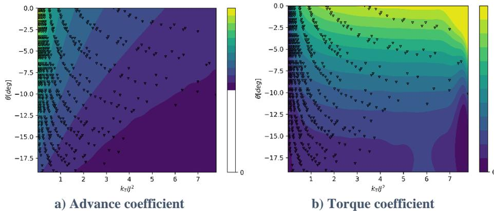
Figure 10: CBT propeller surrogate model response surfaces
