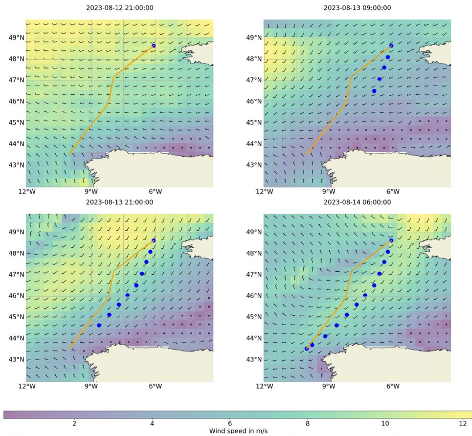
**Figure 23: Trajectories of reference (orange) and optimized (blue) routes in the Biscay scenario for four snapshots. The background map shows wind speed and wind direction as heat map and wind barbs.**
