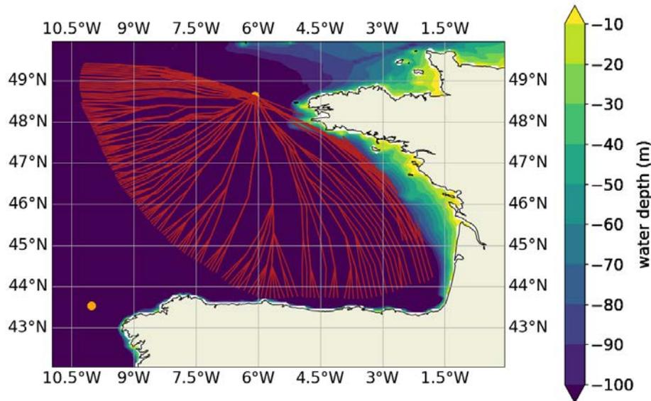
Figure 15: Visualization of route segments at an intermediate routing step of the Isofuel algorithm for a CBT traveling in the Bay of Biscay
