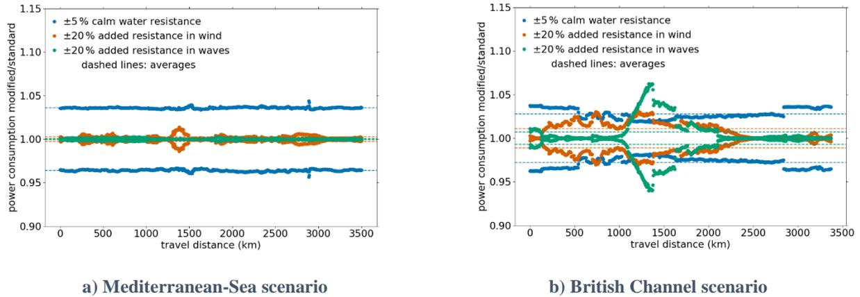
**Figure 22: The ratios for simulations of the power consumption for manipulated resistances over those for standard settings in dependence of the travel distance for historical routes traveled by the CBT**
