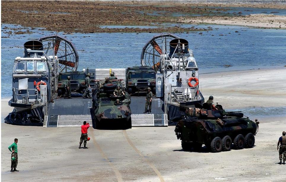
Figure 3: LCAC Unloading (Naval Sea Systems Command, 2021)
