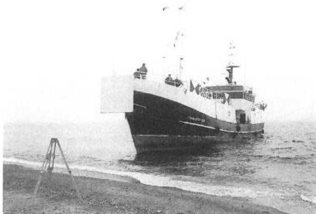
Figure 11: Full Ship Grounding Experiments Conducted by Sterndorff & Pederson (1996)
