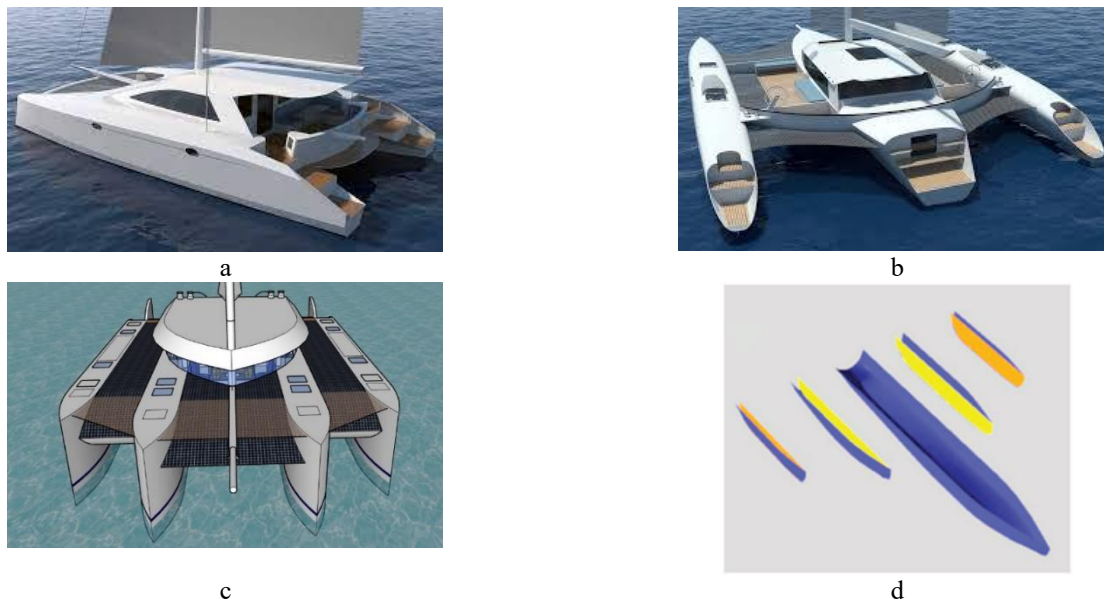
Figure 6. High-speed and low-resistance vessels: (a) Catamaran, (b) Trimaran, (c) Quadrimaran, (d) Pentamaran Ref: (Dr. Hans, 2021; Schionning Designs International (Pty) Ltd, 2024; Yanuar & Waskito, 2017)
