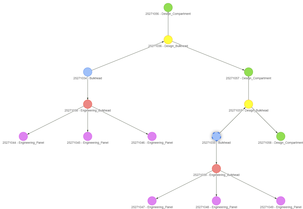
Figure 6: Automatically generated plot of a graph database with two bulkheads and three panels per bulkhead.
