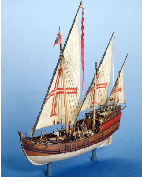
Figure 7 - Three masted caravel with lateen rigged sails (Deutsches Historisches Museum, n.d.-a)
