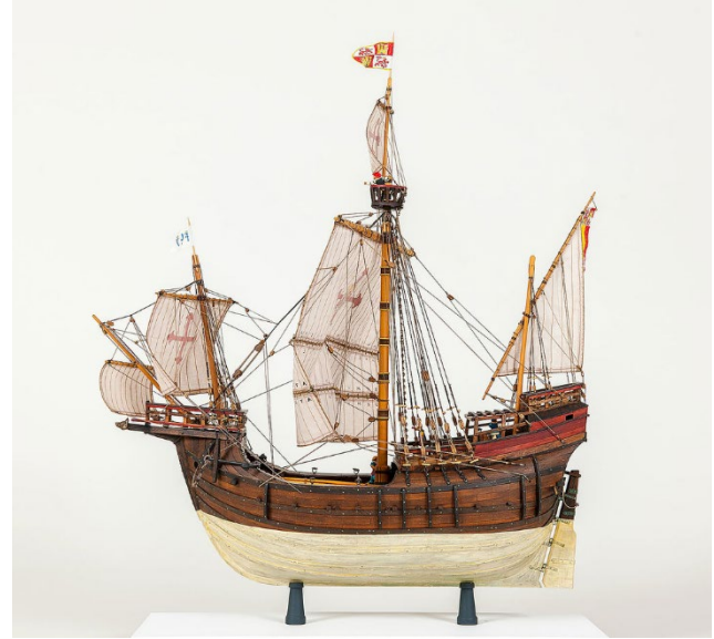
Figure 8 - Three masted carrack / nao with square rigged sails forward and lateen sail aft
