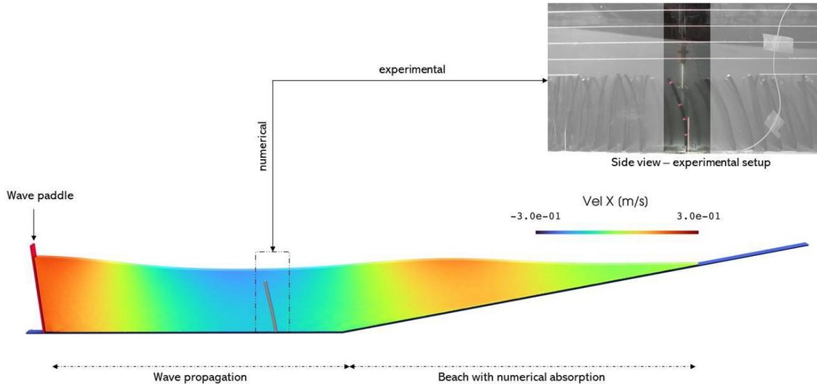
**Figure 1: A composite graphic displaying a side-view snapshot from the laboratory alongside a digital replica (numerical flume) generated using the coupled SPH-FEA model. The horizontal water velocity is plotted using a jet color gradient, while the flexible cylinder is represented in grey color.**
