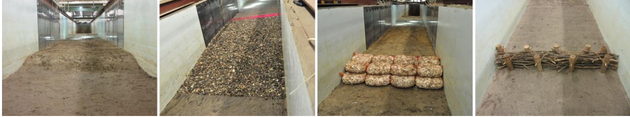
Figure 1. Constructed model edge treatment features from left to right: natural sand edge, rounded gravel berm, oyster-shell filled bag berm, and brushwood dam.
