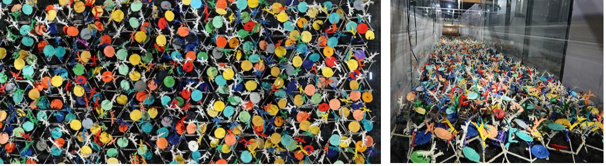
Figure 2. Model scale Reef Star canopy with the largest coral cover attached in plan view (left) and looking down the canopy (right) when installed in the wave flume.
