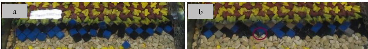
Figure 3. Three rows of cube1- a: after implementing the test of Hs-b: with sacrificial rock- after the test of 1.2 times Hs
