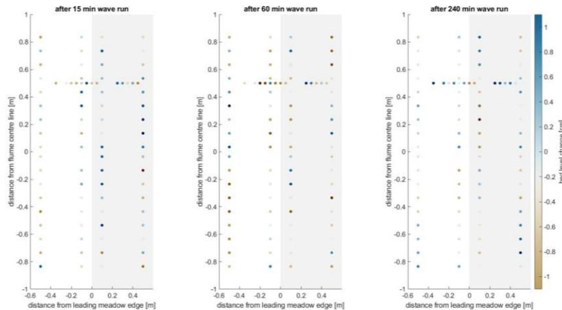
**Figure 1. SEB data on bed level change induced by a wave spectrum ( $H_s = 13$  cm,  $T_p = 2.6$  s). The gray shaded area indicates the artificial seagrass meadow.**
