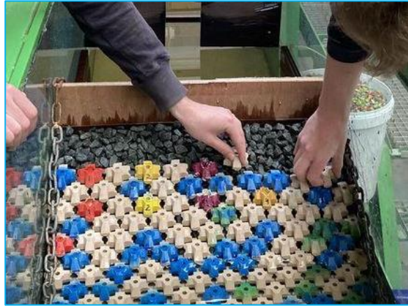
Figure 12. XblocPlus® placement in a wave flume, photo credit DMC.
