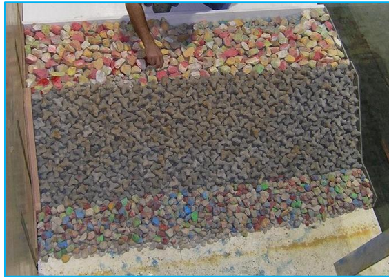
Figure 5. Construction of a breakwater 2D physical model in a wave flume, photo credit ARTELIA.
