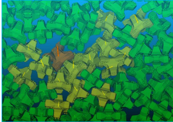
Figure 17. Color-coded display of the block's movements with vectors.
