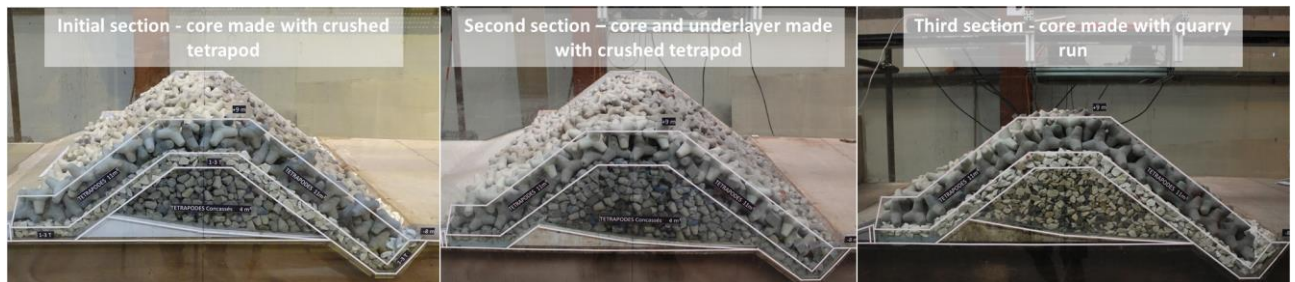
Figure 4. Sections tested in the wave flume. From left to right, SECTION 1, SECTION 2, SECTION 3.
