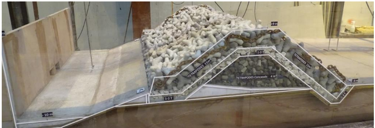
Figure 3. Rubble mound breakwater section + inflow/outflow system in the wave flume – SECTION 1
