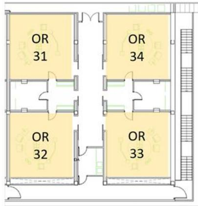
**Fig. 1** - Surgical block No. 3 with four turbulent flow operating rooms.
