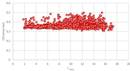
**Fig. 3** - Efficiency Heat vs. Outside Temperature.
