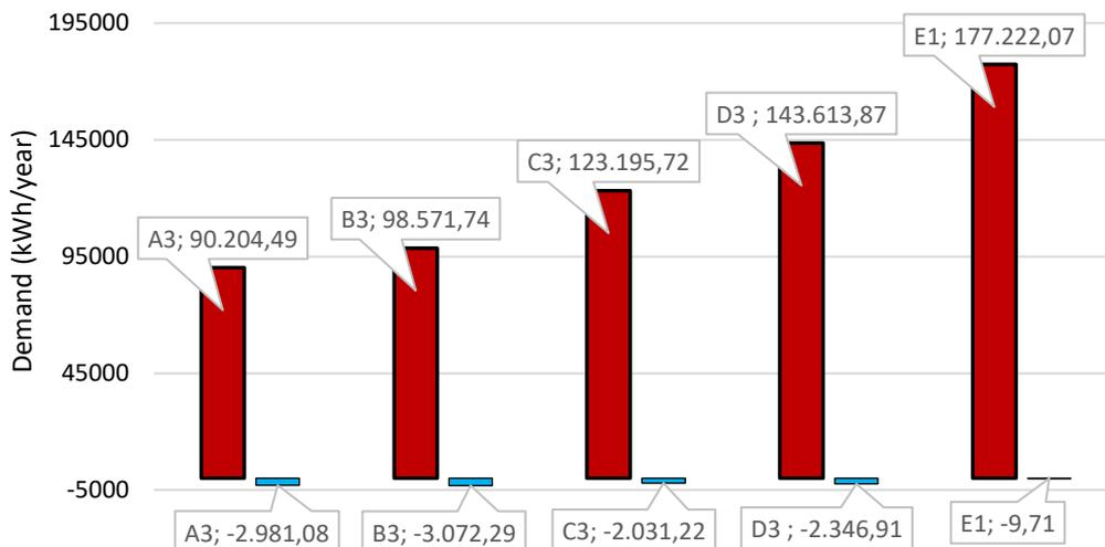
Fig. 6 - Heating and cooling demands for different climate zones.
