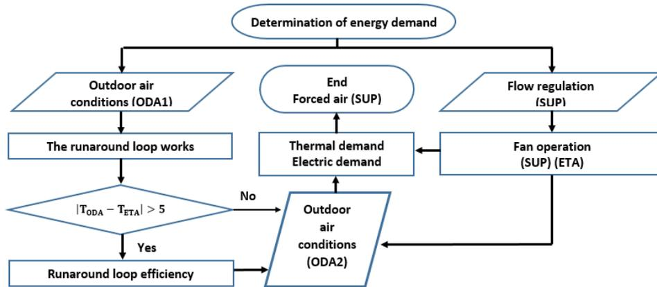
Fig. 5 - Flow chart used to determine thermal and electrical energy demand.
