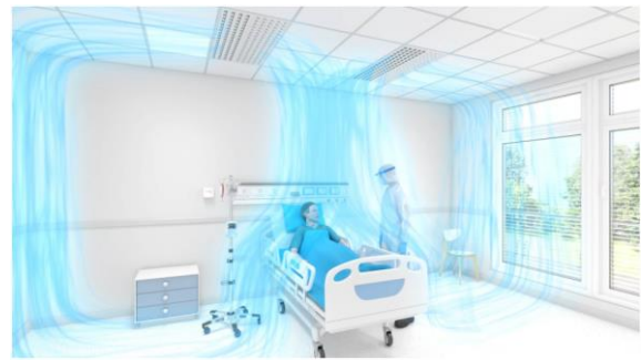
Fig. 5 - Protective airflow system concept, Isolation room. /10/
