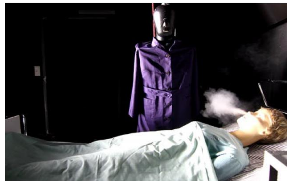
Fig. 9 – Patient outbreak with protective airflow pattern in isolation room at 200 l/s flow rate.
