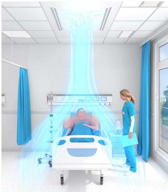
Fig. 4 - Protective airflow system concept, patient room. /10/
