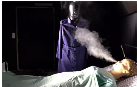
Fig. 7 – Patient outbreak with protective airflow pattern in isolation room at minimum 30 l/s flow rate.
