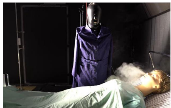
Fig. 8 – Patient outbreak with protective airflow pattern in isolation room at 70 l/s flow rate.
