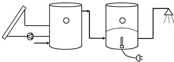
**Fig. 3** – Diagram of the thermal solar system with electric boiler.
