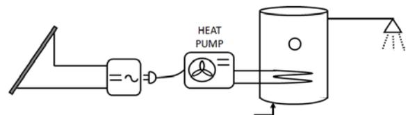
**Fig. 6** – Diagram of the photovoltaic system with heat pump.
