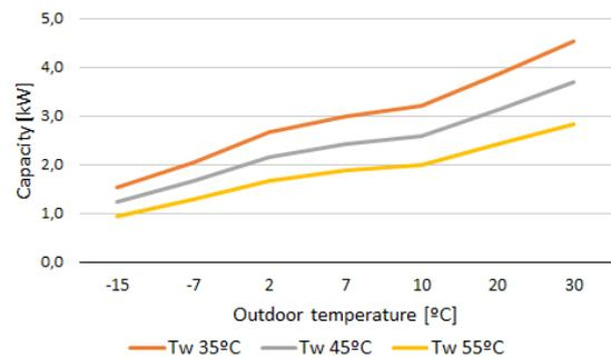
**Fig. 5** – Heat pump capacity.
