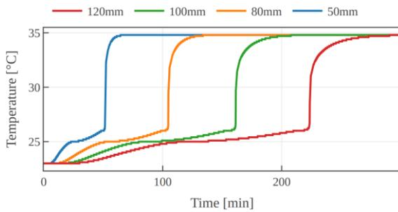
**Fig. 13:** Temperature inside the storage tank in time during the process of charging.
