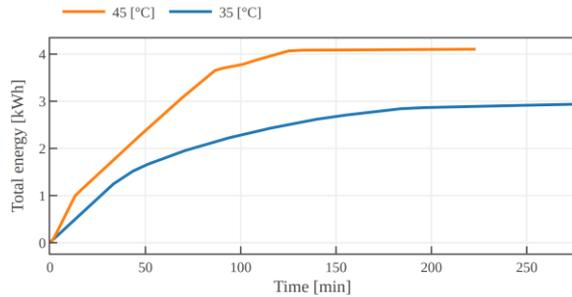
**Fig. 9.** Heat released during discharging of LHS.
