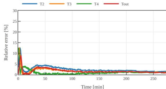
**Fig. 10:** Relative errors between simulation and measuring results during the process of charging with inlet temperature of 35°C.
