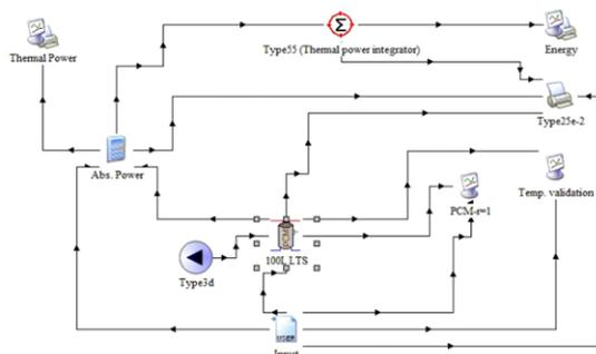
**Fig. 10:** Schematic of simulation system TYPE 840 in the Trnsys software environment.
