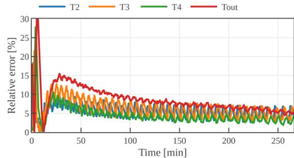
**Fig. 10:** Relative errors between simulation and measuring results during the process of discarding.
