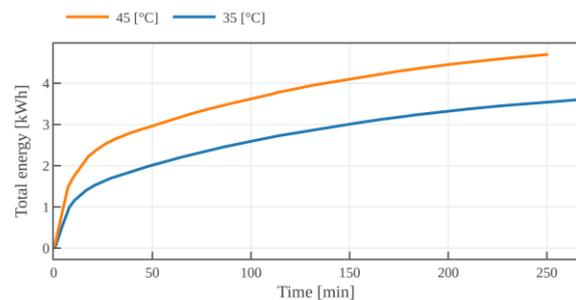
**Fig. 7.** Storage energy in different charging temperature of 35 and 45 ° C.
