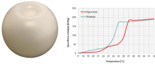
**Fig. 2:** Spherical modules filled with PCM and enthalpy-temperature function of PCM of FSS PCM HS24.
