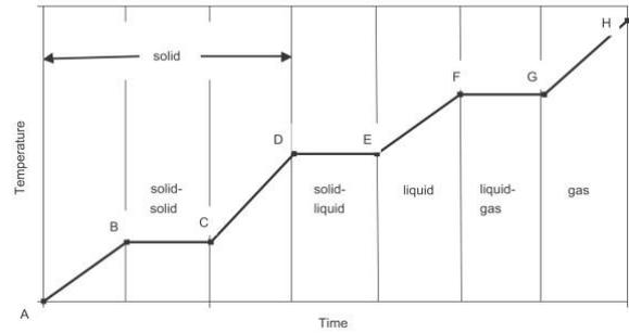
**Fig. 1:** Temperature-time diagram for the heating of substance(9).
