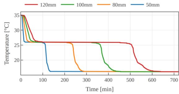
**Fig. 15:** Temperature inside the storage tank in time during the process of discharging.
