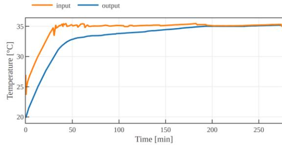
**Fig. 5** Charging of LTS with inlet temperature of 35° C.
