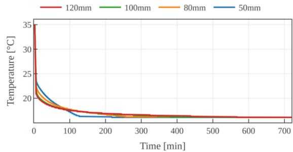
**Fig. 16:** Outlet temperature during the process of discharging.
