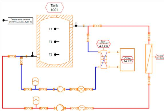
**Fig. 4:** Scheme of experimental setup.
