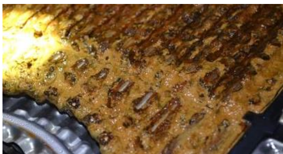
Fig. 6 Fouling layer on a heatexchangerplate
