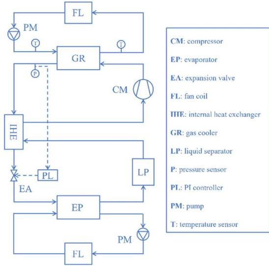
**Fig. 1** – CO<sub>2</sub> heat pump experimental setup
