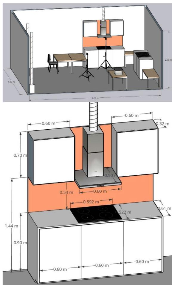
**Fig. 1** - Upper: Kitchen lab dimensions and layout. Lower: Kitchen setup.
