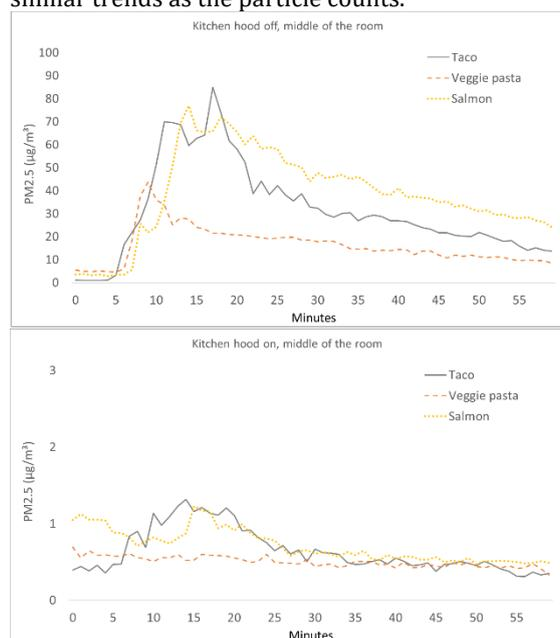
**Fig. 9** - PM<sub>2.5</sub> mass concentrations measured in the middle of the room, for the three different meals. Upper: with kitchen hood off, and lower: with the kitchen hood on.
