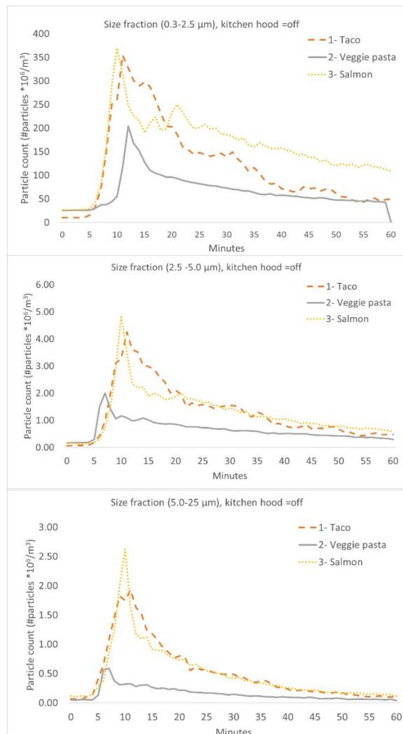
**Fig. 4** - Particle counts for the three test meals with the kitchen hood off according to different size fractions. Measurement location=breathing height of the cook. Note the different scale on the y-axis.
