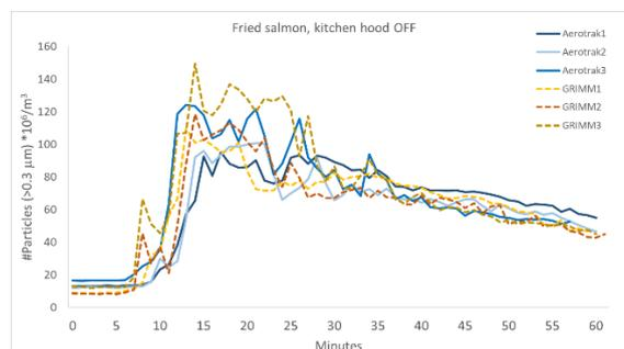
**Fig. 3** - Particle counts as measured by GRIMM and AeroTrak at location 2 (middle of the room) cooking meal 3 – fried salmon when the kitchen hood was turned off.
