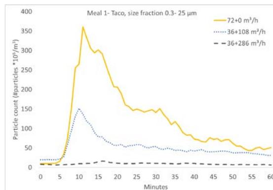
**Fig. 6** - Particle counts for all size fractions  $0.3\text{-}25 \mu\text{m}$  (averaged) for meal 1 - taco at different ventilation rates. Measurement location =breathing height of the cook. The cooking time is 16 minutes.
