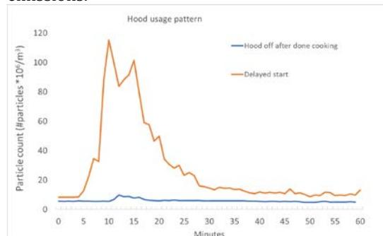
**Fig. 8** - Particle counts for all size fractions for meal 1-taco with different hood usage patterns.
