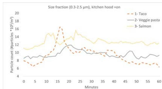
**Fig. 5** - Particle counts for the smallest size fraction  $0.3\text{-}2.5 \mu\text{m}$  (average values) for the three test meals with the kitchen hood on medium setting ( $36+286 \text{ m}^3/\text{h}$ ). Measurement location =breathing height of the cook.
