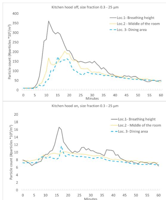
**Fig. 7** - Particle number concentration (0.3-25 µm) for Meal 1-taco in all three locations (upper with the kitchen hood off, lower with the kitchen hood on).
