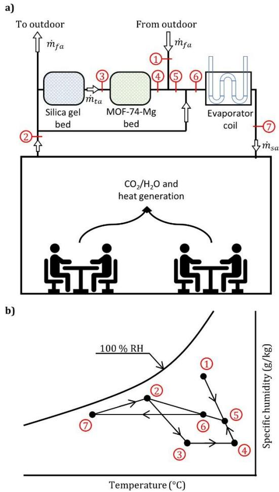
**Fig. 1** – Schematic of a) the proposed ventilation system and b) the psychrometric process of the supply airflow.
