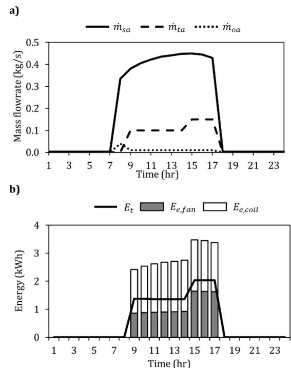
Fig. 2 – The hourly variation of a) the system's operating parameters and b) the corresponding electrical and thermal energy consumptions.
