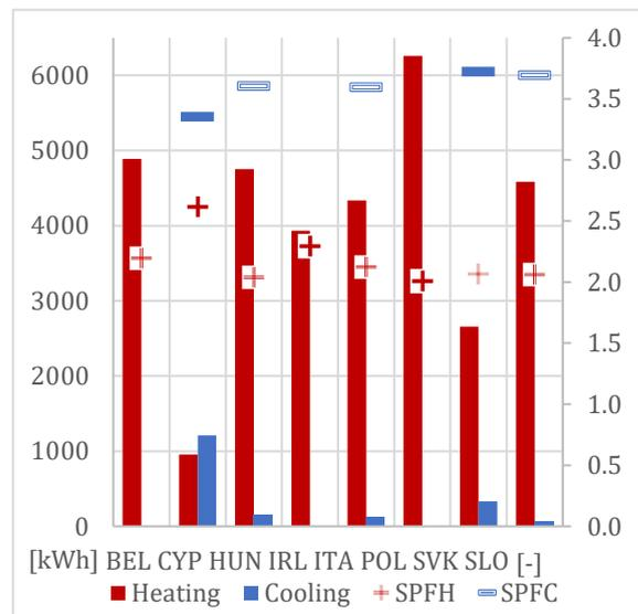
**Fig. 5** - Seasonal performance factors of heating and cooling and energy consumptions
