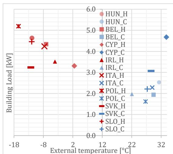
Fig. 2 – Net energy demands and loads of the reference building in different Member States.
