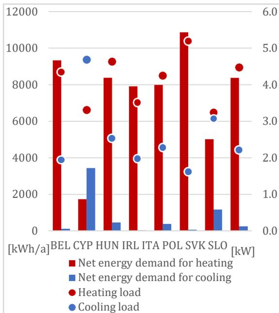
**Fig. 4** - Net energy demands of the reference house for the test reference year of each countries.
