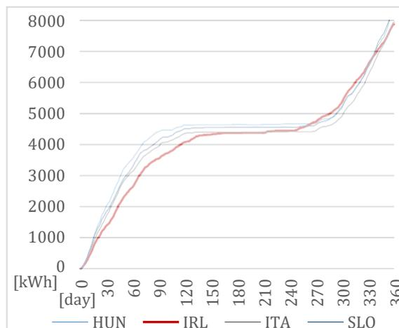
Fig. 3 – Accumulated heat loads of the countries with similar heating demand.
