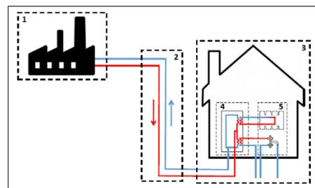
**Fig. 1** - A simplified illustration of a district heating system, where 1 represents production, 2 represents distribution, 3 represents the customer installations, 4 represents the customer substation, and 5 represents the internal heating system.
