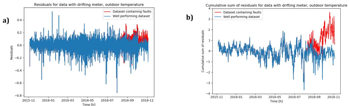
**Fig. 6** – Analysis of the residuals between the real and the predicted values for the data set without a fault (blue line) and the data set with a drifting outdoor temperature meter (red line). **a)** Residuals between real and predicted values as a function of time. **b)** Cumulative sum of residuals as a function of time.
