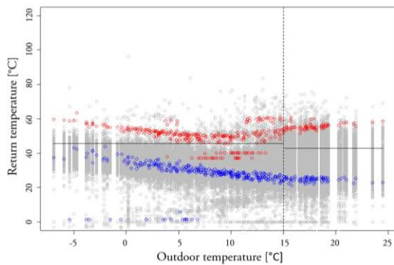
**Fig. 4** - Return temperature signature with one well performing (blue circles) and one poorly performing (red circles) installation represented.
