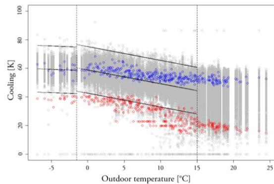
**Fig. 3** - Cooling signature with one well performing (blue circles) and one poorly performing (red circles) installation represented.
