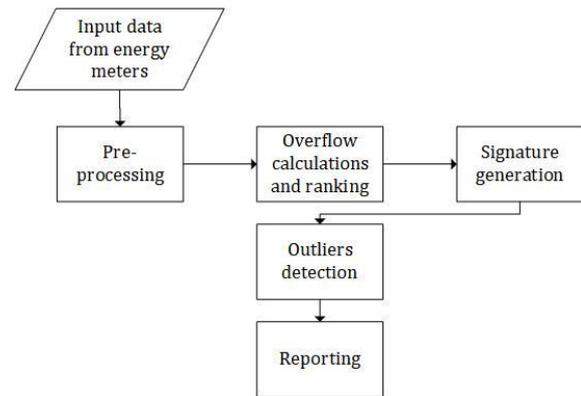
**Fig. 2** – Schematic view of the cluster-based fault detection method.
