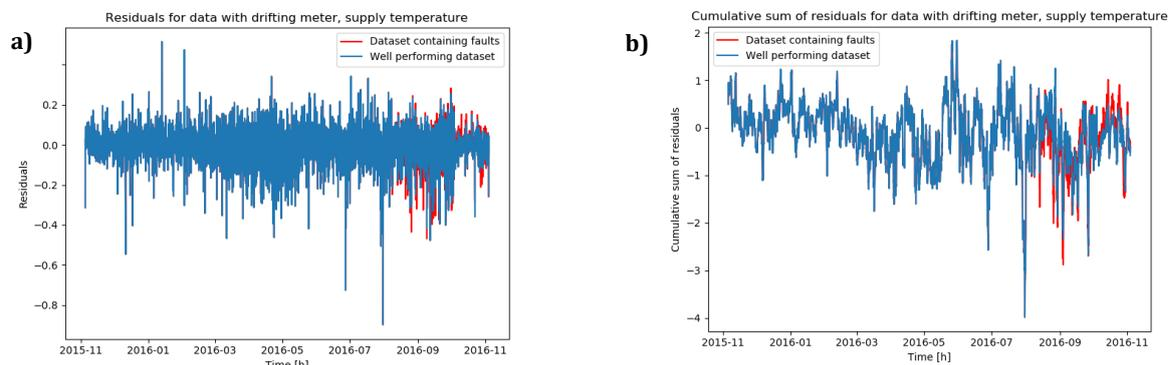
**Fig. 7** – Analysis of the residuals between the real and the predicted values for the data set without a fault (blue line) and the data set with a drifting supply temperature meter (red line). **a)** Residuals between real and predicted values as a function of time. **b)** Cumulative sum of residuals as a function of time.
