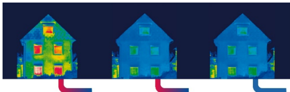
Fig. 2 - Illustration of the thermal development in building technology as an infrared thermography.
