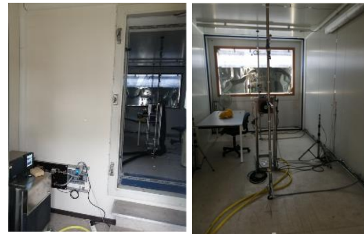
Fig. 4 - Heating/Cooling systems, left: Generation - Thermal bath, right: View of inside the Passys Cell
