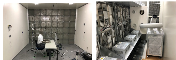
(1) Thermal manikin in the chamber (2) Fan room Photo. 1 Climate chamber experiment
