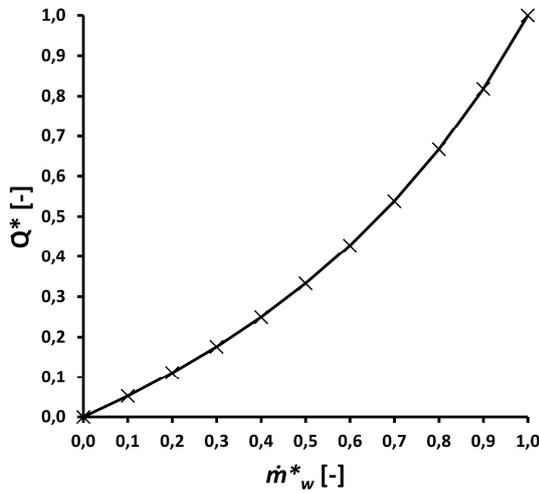
**Fig. 7** - Heat exchanger characteristic for a cooling coil with a decreasing CHWdT in part load
