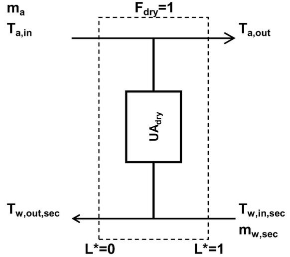
Fig. 3 - Model and energy balance of a dry cooling coil in counter flow
