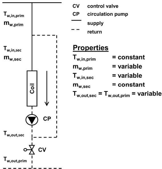
Fig. 2 - Hydraulic configuration of a cooling coil, mixing circuit (module 5) [17]
