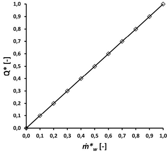
**Fig. 6** - Heat exchanger characteristic for a cooling coil with a constant CHWdT in part load
