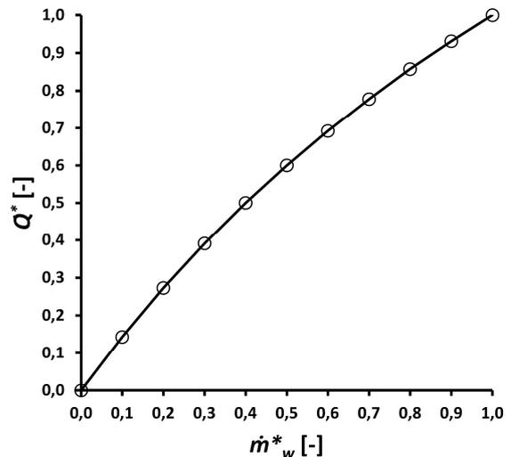
**Fig. 5** - Heat exchanger characteristic for a cooling coil with an increasing CHWdT in part load
