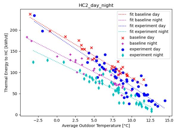
**Fig. 6** – Energy KPI with day/night split for the HC2 riser with 14 radiators over 30 days of baseline and 69 days of experiment
