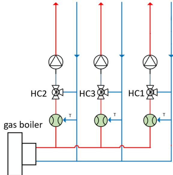
**Fig. 3** – Building heat generation and distribution layout showing three heating circuits (HC2, HC3 and HC1 from left to right).
