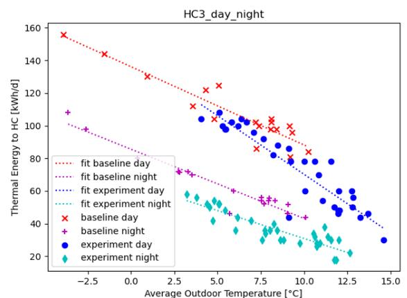
**Fig. 7** – Energy KPI with day/night split for the HC3 riser with 5 radiators over 19 days of baseline and 56 days of experiment
