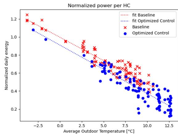
**Fig. 5** – Normalized energy results for the whole building (i.e. Energy of HC1, 2 and 3 are normalized at 0°C outdoor temperature, in reference to the baseline, and aggregated)
