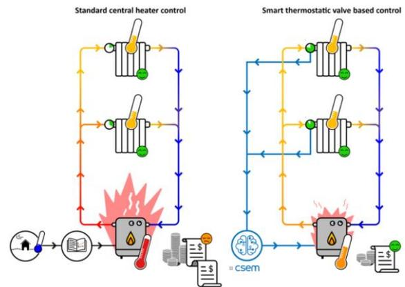
**Fig. 1** – Standard central heater control (left), STV based data-driven heat control (right)
