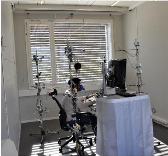
**Fig. 2** – Photo of the experimental setup and placement of comfort stands (S window with direct solar exposure, the office desk behind the calorimeter stand)
