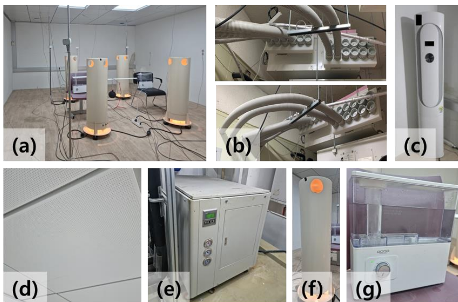
Fig. 4 – Experiment facilities. (a) indoor chamber. (b) HPDC system. (c) PAC system. (d) RCP. (e) chiller for RCP. (f) 60W light bulb dummy for sensible load trace. (g) 157W humidifier for latent load trace.
