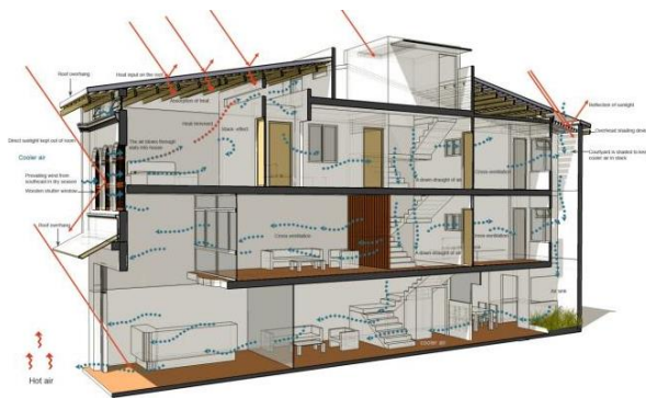
Fig 21 - Climatic responsive design of house 111 in the renovated case in daytime
