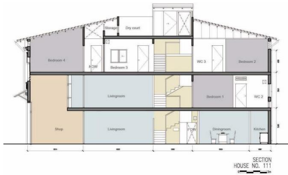
Fig 6 - Floor plans and section of House No.111
