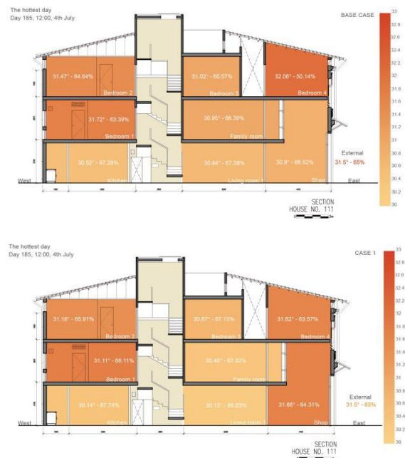
Fig 11 - Thermal performance in two cases - base case (above): without ventilation, case 1 (below): with ventilation
