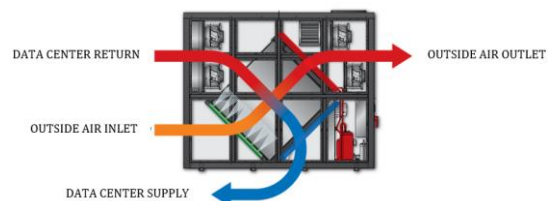
Fig. 4 – Indirect evaporative cooler principle scheme
