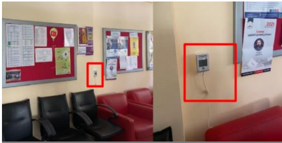
Fig. 2 - Placement of Testo 160 Indoor Air Quality (IAQ) Data Logger
