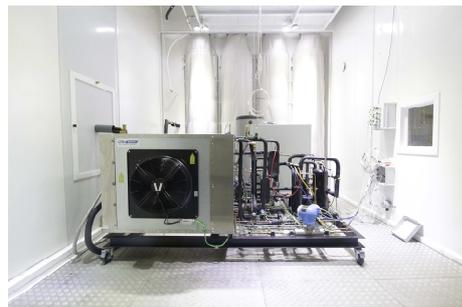
**Fig.3** - DSHX test bench installed inside the climatic chamber.
