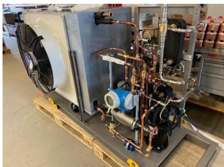
**Fig. 21** – Second prototype of the DSHP.
