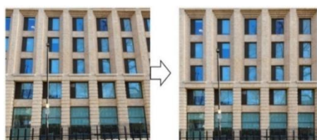
Fig. 2 - An example of rectified images (left: tilted images, right: rectified images)
