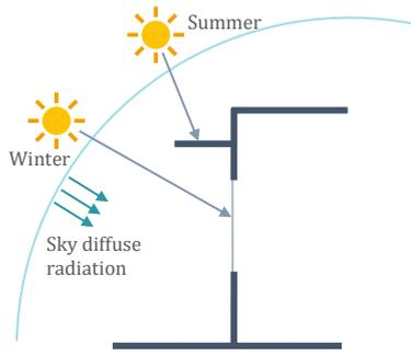
**Fig. 5** – Fixed solar protection.
