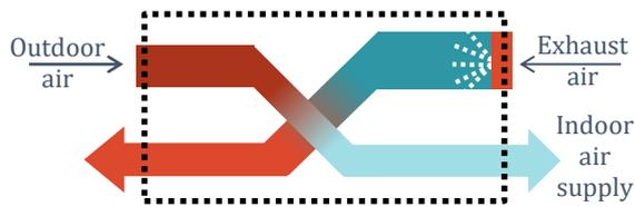
**Fig. 6** – Schematic of an Indirect Evaporative Cooler.
