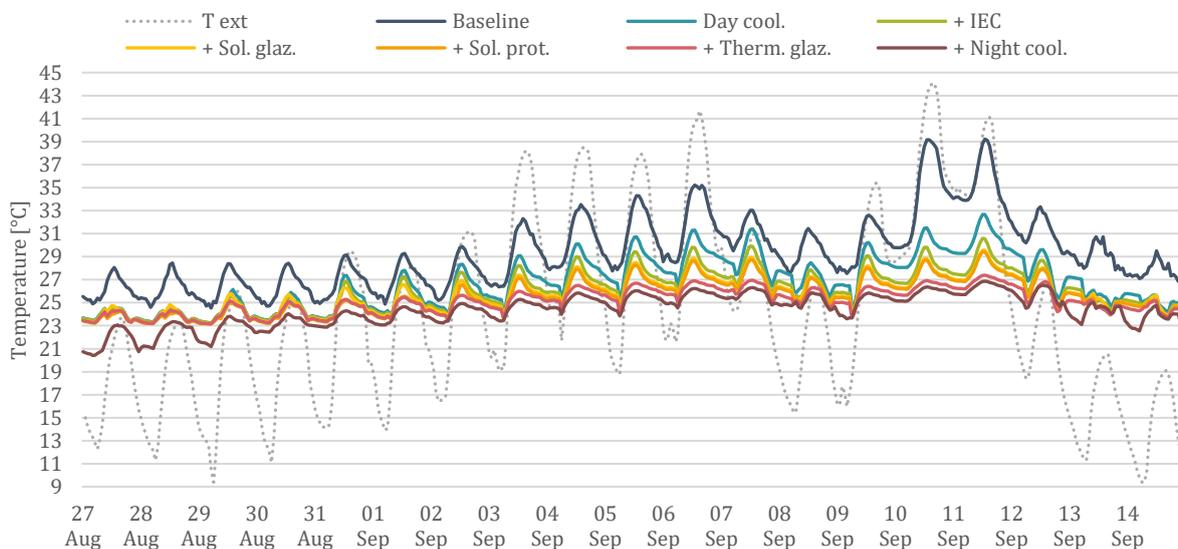
**Fig. 8** – Evolution of the indoor temperature during a heat wave considering passive cooling techniques.
