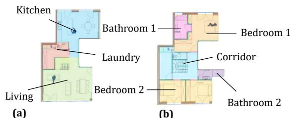
**Fig. 2** – Upper view of the duplex (a) first floor (b) second floor and division in thermal zones.
