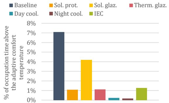
**Fig. 7** – Impact of passive cooling techniques on overheating risk.
