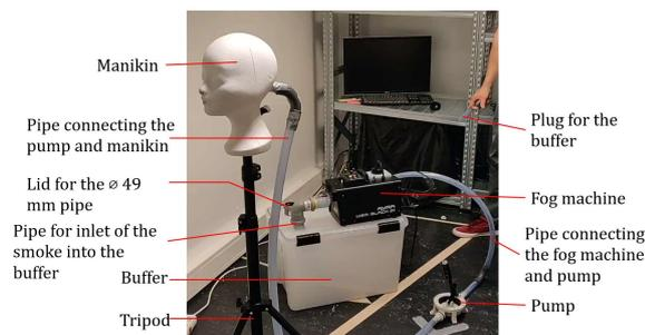
Fig. 1 – Setup of the portable fog generator.
