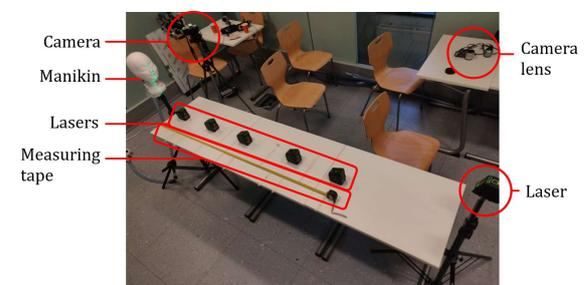
Fig. 3 – Setup of the airflow pattern visualisation experiment.
