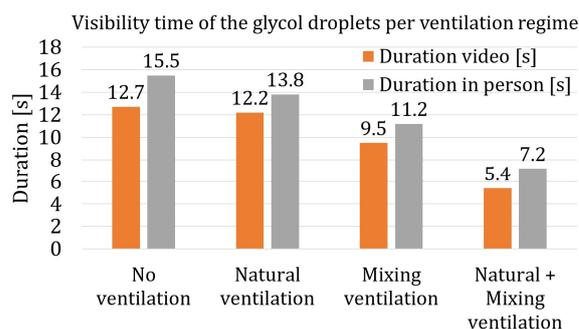
**Fig. 5** – The droplets settled or evaporated faster in the recordings than with the naked eye. Increasing the indoor air velocity decreases the visibility of the droplets.
