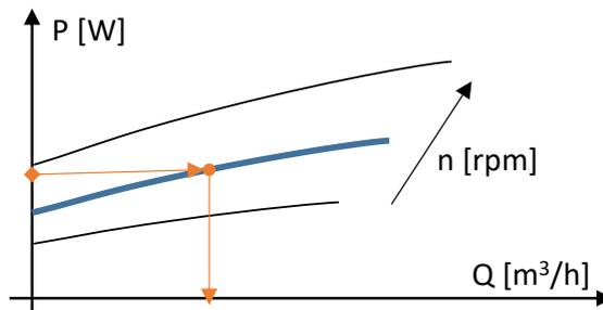
**Fig. 2** – The basic principle of inferring flow from a pump electrical power reading.
