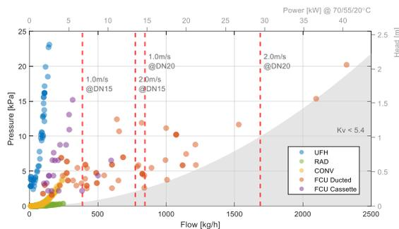
**Fig. 4** – Typical design operation conditions for underfloor heating (UHF), radiators (RAD), convectors (CONV) and fan-coil units (FCU). All datasheet values normalised to conditions 70/55/20°C using the norm EN 442-1:1995
