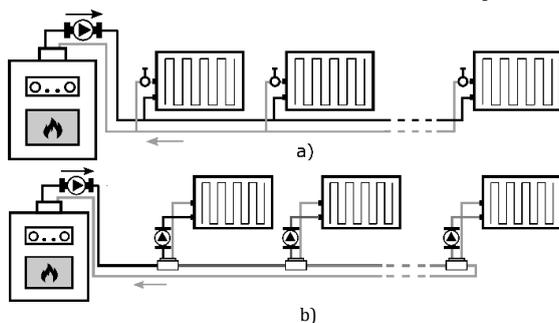
**Fig. 1** – Hydronic system topologies: a) two-pipe throttling system, b) pumping one-pipe system.
