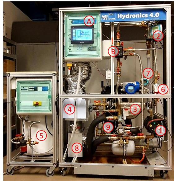
**Fig. 8** - Hydronic Testbed. A) Testbed controller, B) One-pipe control pump device, 1) Primary pump, 2) Primary induction flowmeter, 3) Secondary Coriolis flowmeter, 4) Water-to-air heat exchanger, 5) Main tank, 6) Actuated valve, 7) Differential pressure sensor, 8) Controlled fan, 9) Second tank for sudden temperature steps.
