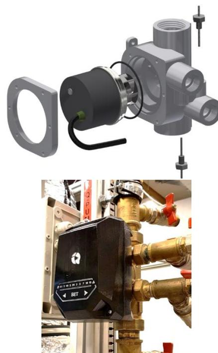
**Fig. 5** – One-pipe control pump device. Early design at the top (3D print manufacturing); brass-casted and machined final design with injection-mould-manufacturable electronics cover on the bottom.
