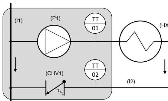
**Fig. 3** – One-pipe control pump device scheme. HX – heat exchanger, CHV – check-valve, I – pipe, P – pump, TT – temperature sensor.
