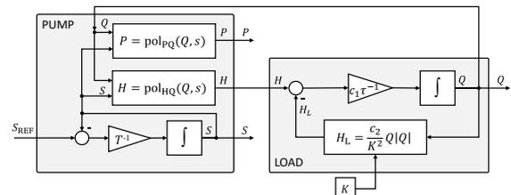
**Fig. 7** – Simplified scheme of the dynamical model used for mass flow estimation.
