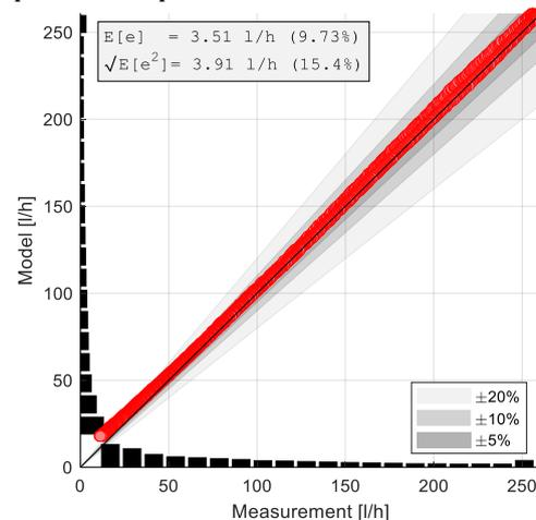
**Fig. 9** - Flow estimation precision for a random fixed position of the actuated valve in the secondary circuit.
