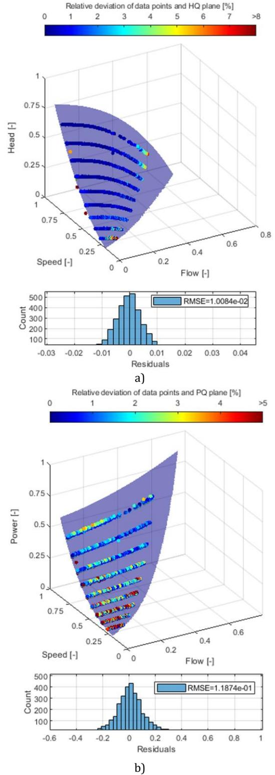
**Fig. 6** – IQP device characteristics fitting: a) HQ plane, b) PQ plane.
