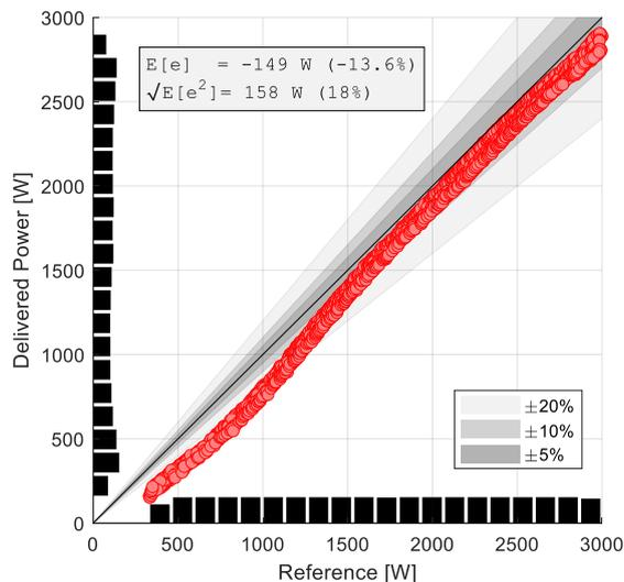
**Fig. 10** – Steady-state heat flow control precision for the heat terminal present at the hydronic testbed.
