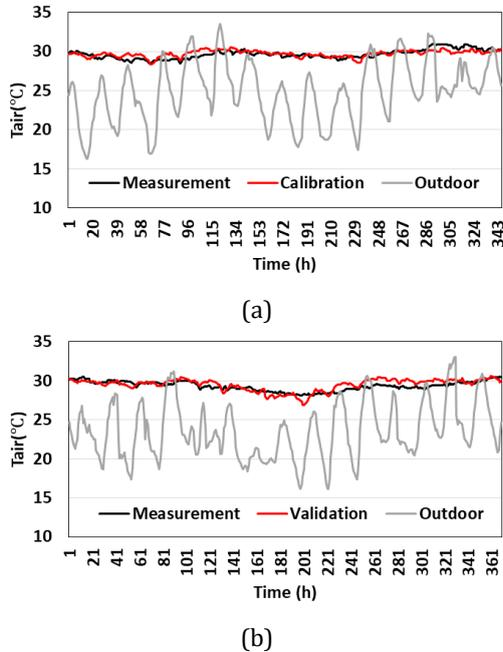
**Fig. 4** - Comparison of the measured and simulated data (room averages of LTCB) during (a) calibration period and (b) validation period
