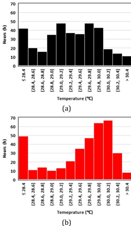
**Fig. 5** - Distribution of average room data of LTCB during the validation period: (a) measured and (b) simulated temperatures
