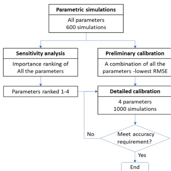
Fig. 3 - Building calibration procedure
