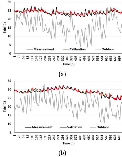
**Fig. 6** - Comparison of the measured and simulated data (room averages of PS) during (a) calibration period and (b) validation period
