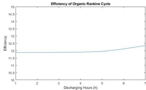
Fig 6. Efficiency of Organic Rankine Cycle according to discharging hours
