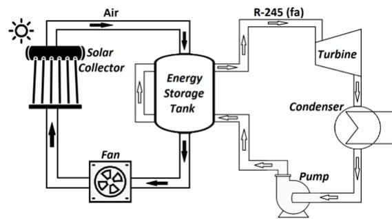
**Fig. 1. Schematic of the simulated system**
