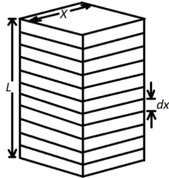
Fig. 3. The discretized view of the tank
