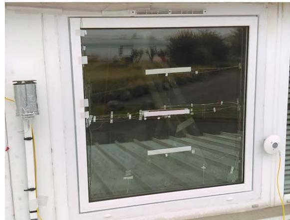
**Fig. 2** Instrumented window on the south façade of a faculty building in Bethune
