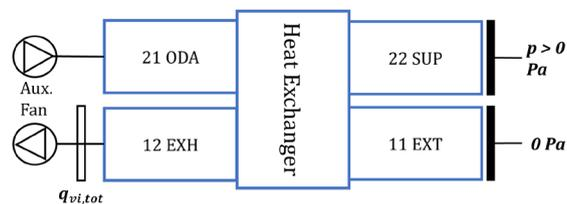
Fig. 1 - Test setup for Pressure Method
