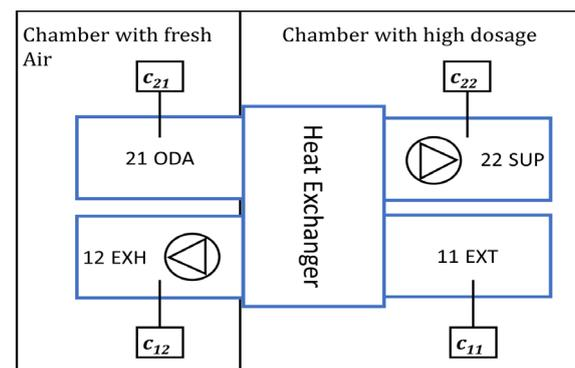
Fig. 3 - Test setup for Chamber Method
