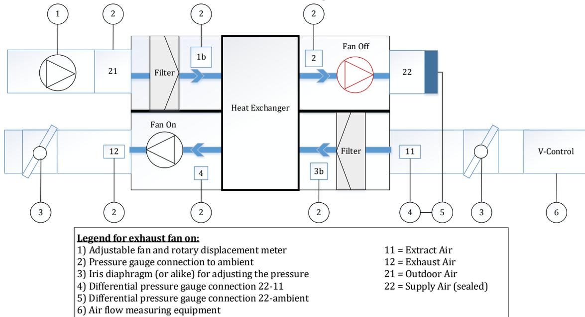
Fig. 6 - Test setup APM
