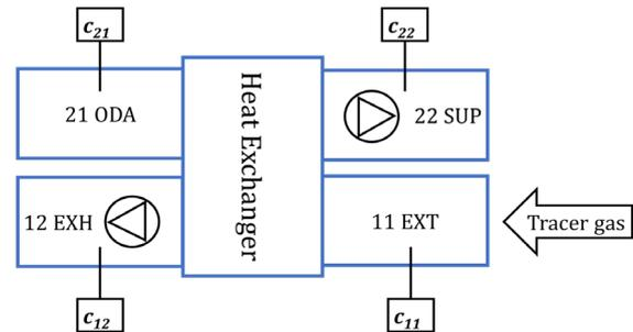
Fig. 2 - Test setup for In-duct Method
