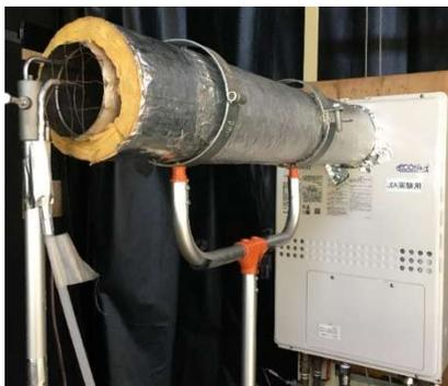
Figure3. Experimental method for blowout condition of Exhaust port
