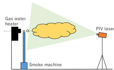
Figure5. Experimental method for visualization of exhaust
