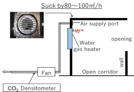
Figure2. a gas water heater and an air supply port installed in an open corridor
