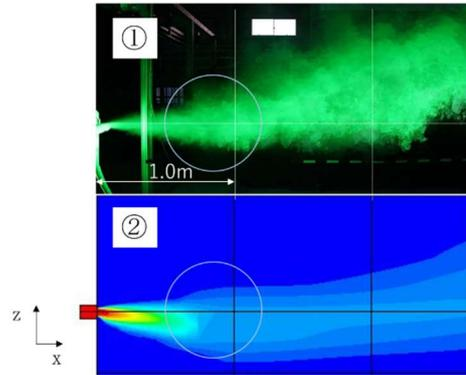
Figure 12. difference in center height of the exhaust orbit(①: results of visualization experiments, ②: analysis results)
