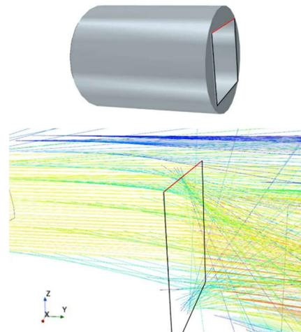
Figure13. Velocity vector diagram near exhaust model
