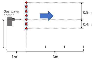
Figure4. Experimental method for exhaust distribution
