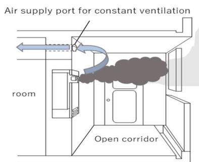
Figure1. Installation status of gas water heaters in Japan
