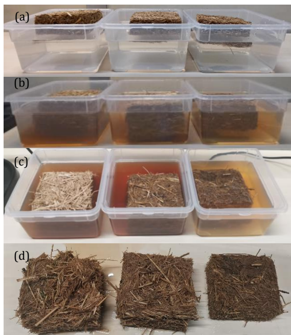
Fig. 3 - From left to right: sample 1, 2 and 7 immersed in water for (a) 1 min; (b) 1 h; (c) 24 h and (d) after 24h.
