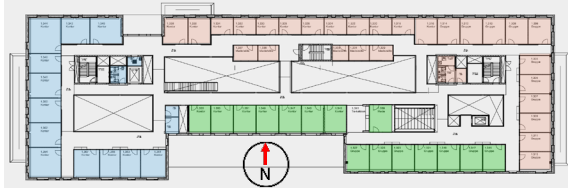
Fig. 5 - Thomas Manns Vej 23, 3 rd floor coverage by AHUs, the blue area is covered by the AHU used in this paper.
