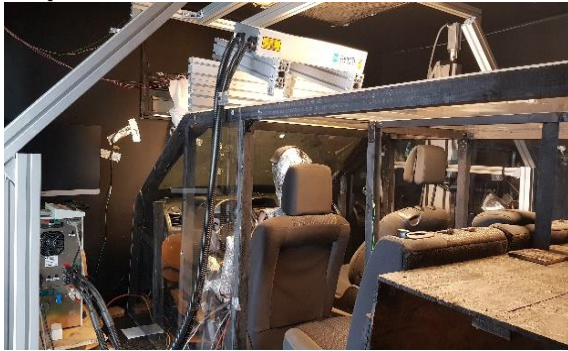
Fig. 1 – Experimental setup – 1:1 scale cabin mock-up with transparent walls.
