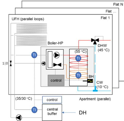
**Fig. 4** – Simplified hydraulic scheme of a booster heat pump.
