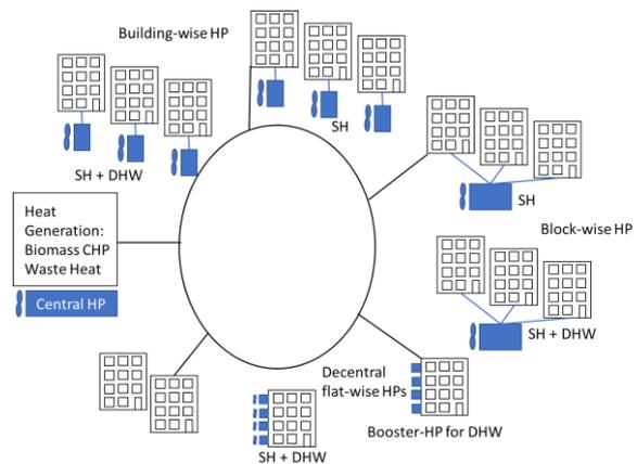
**Fig. 3** – Sketch of possible solutions for HP integration (in blue) in a DH system.
