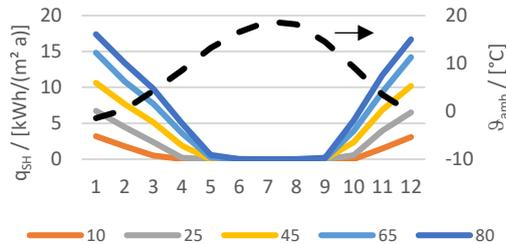
**Fig. 2** - Monthly space heating demand of the building with different qualities of the envelope in kWh/(m<sup>2</sup> a), considering the climate of Innsbruck (site climate acc. to OIB-6\_2019)
