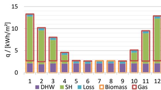
**Fig. 7** - Reference DH system with 40 % biomass and 60 % gas.
