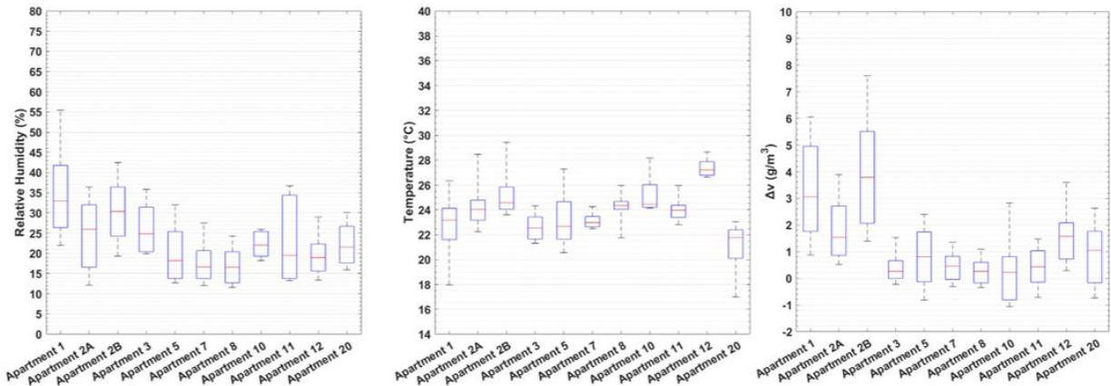
**Fig. 6** - Measurements of RH, air temperature and  $\Delta v$  values from the living room of each tested apartment.
