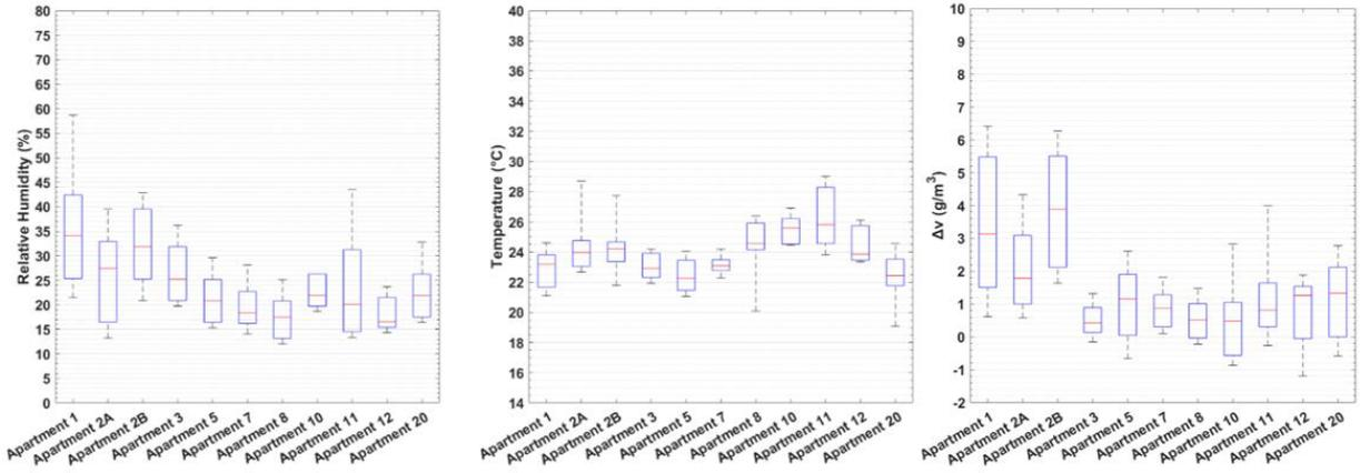
Fig. 5 - Measurements of RH, air temperature and  $\Delta v$  values from the kitchen of each tested apartment.
