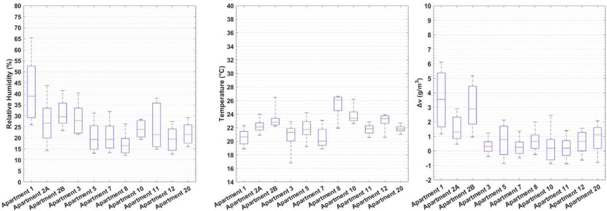
Fig. 7 - Measurements of RH, air temperature and  $\Delta v$  values from the master bedroom of each tested apartment.
