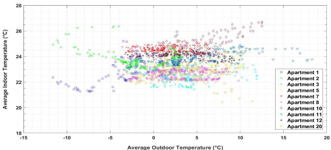
Fig. 1 - The correlation between indoor and outdoor temperatures, average values per house [6].
