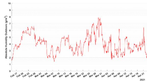
Fig. 2 - Absolute humidity outdoors expressed in g/m<sup>3</sup>, during the experiment period [6].
