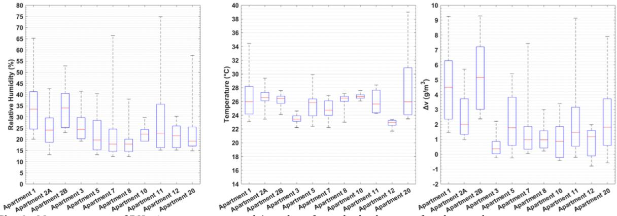
Fig. 4 - Measurements of RH, air temperature and  $\Delta v$  values from the bathroom of each tested apartment.
